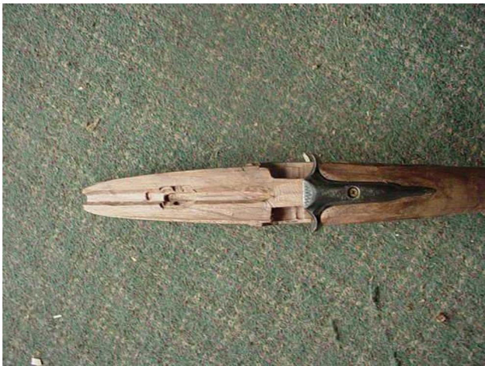
Ok now here I jumped ahead and inlet the barrels with breach into the stock, I then cut out the breach hooks and fit them to the standing breech and inlet the standing breach, before doing a rough shape of the stock.
