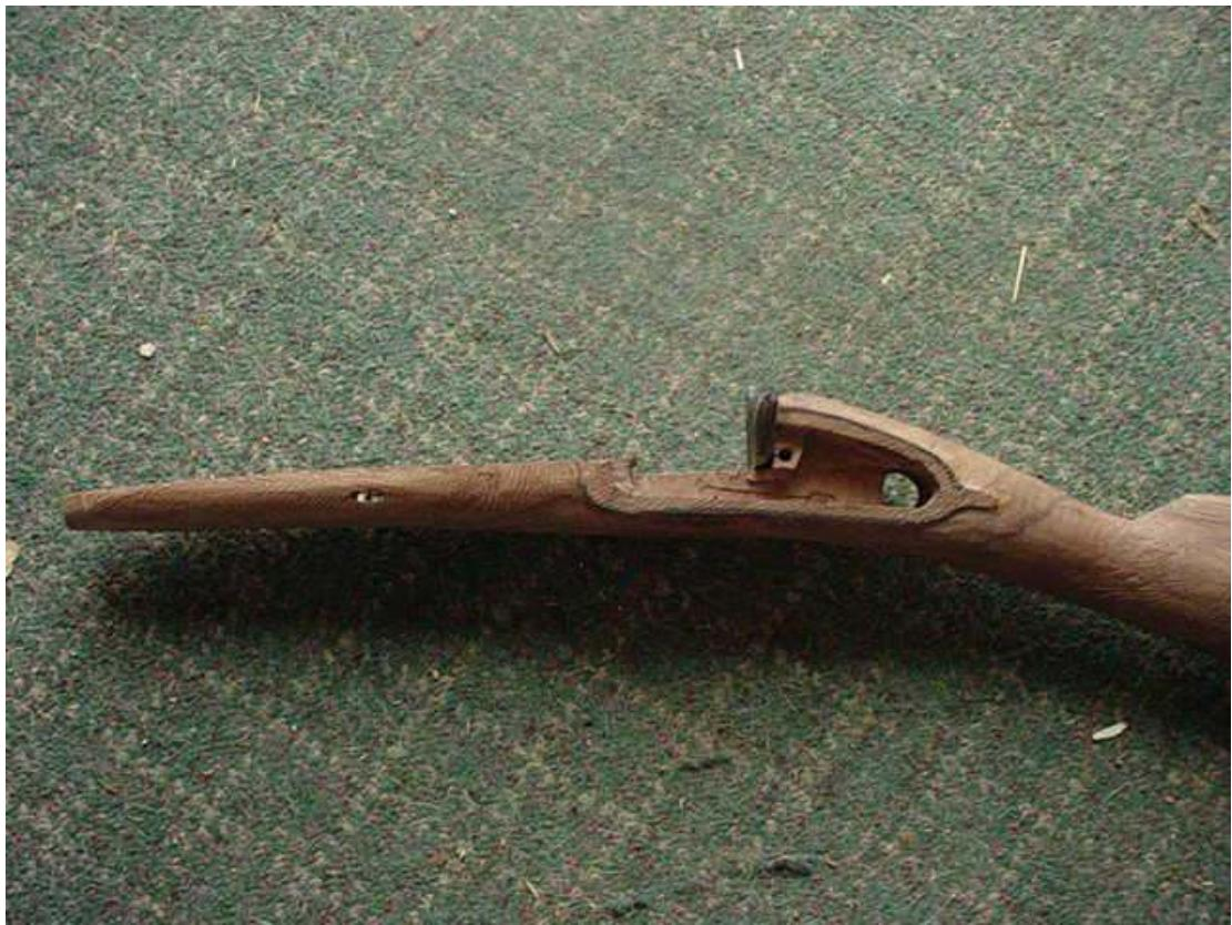
Ok so now once the locks were inlet and the sear whole drilled we set the locks in to check the fit and alignment to the breach plugs in this photo you will see I have outlined the area to grind out for the nipple seats . The locks are aligned and hammers are setting on the tumblers but not screwed on ...
