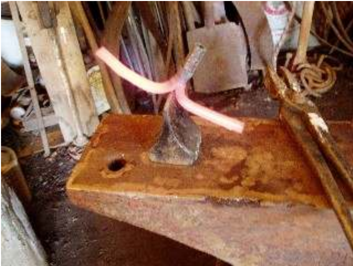
Hot split opened to forge out the tines
