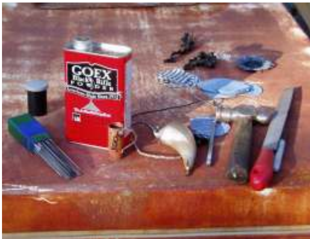
300 gr. Copper Powder Measure, Priming Horn, Patches, and Instruments of sight adjustment. Note: .024" pillow ticking was not heavy enough and yield the totally blown out and burnt patches. Heavy jean was the proper weight cloth and a shot patch verified that.
