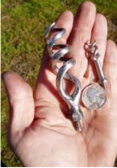
Finished hand forged gun worm for the Wall Gun the small one is a cast (from The Rifle Shoppe) that I finished up, for .40-.50 cal.
