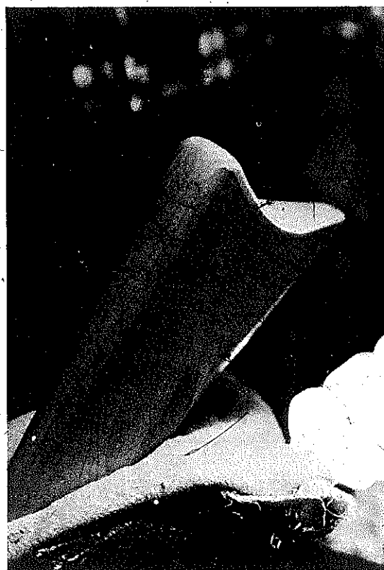
PLATE 293 The butt of the stock after it has been rasped down.
