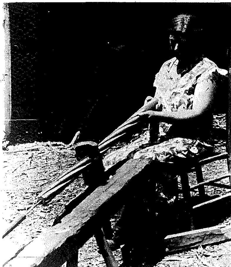
PLATE 186 An old photograph of a mountain woman named Mary Owensby rifling a barrel. (By permission of the Doris Ullman Foundation and Berea College.)
