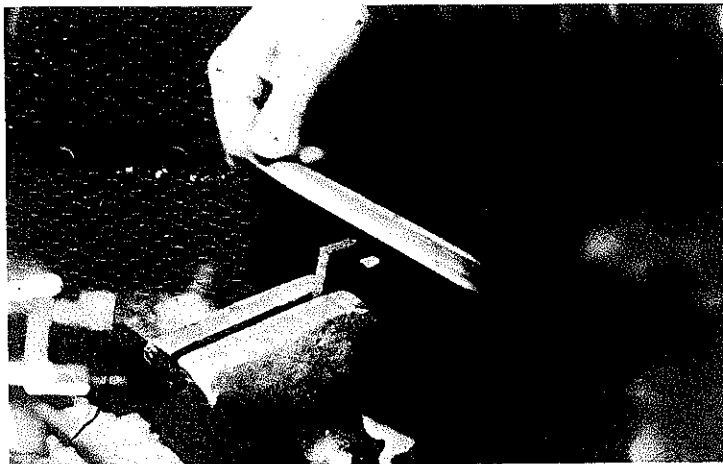
PLATE 276 The trigger blank was one quarter inch thick. As this is much too thick for the final product, except for the trigger pad itself, he rasps about one eighth of an inch off each side, scoring it with a hacksaw to make the rasping easier.
